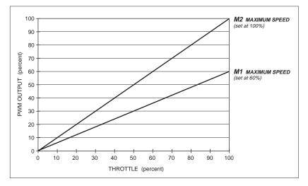
The speed interlocks (see Section 4) ensure that Mode 2 is by definition the faster of the two modes. The M1 Maximum Speed cannot be set higher than the M2 Maximum Speed.
