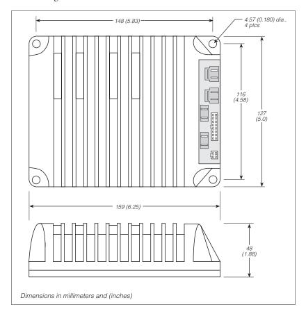
The 1225/35 controller can be oriented in any position. To ensure full rated output power, the controller should be positioned so that the maximum available airflow travels across its ribs. Fasten the controller to a secure mounting bracket or other surface, using the four mounting holes provided. Be sure to allow easy access to the controller's connection face so that the 1307 handheld programmer can be plugged into the controller after it is installed.
