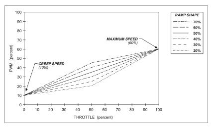
In all cases, the ramp shape number is the PWM output at half throttle, as a percentage of its full range. In Figure 24, for example, the 50% ramp shape gives
