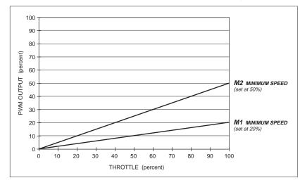
The speed interlocks (see Section 4) ensure that the minimum speed is set lower than the maximum speed in each mode (M1 Min Speed < M1 Max Speed, and M2 Min Speed < M2 Max Speed).
