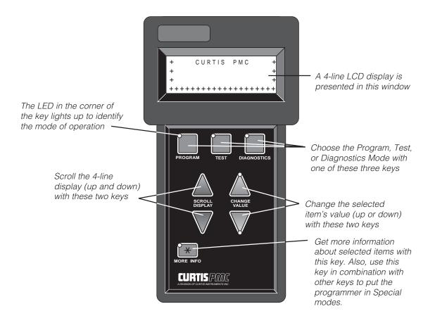
The programmer is operated via an 8-key keypad. Three keys select operating modes (Program, Test, Diagnostics), two scroll the display up and down, and two change the values of selected parameters. The eighth key, the MORE INFO key, is used to display further information about selected items within any of the three standard modes. In addition, when pressed together with the PROGRAM or the DIAGNOSTICS key, the MORE INFO key selects the Special Program mode or the Special Diagnostics mode.
