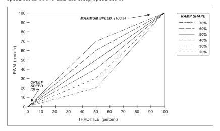
Changing either the maximum speed setting or the creep speed setting changes the output range of the controller. Ramp shape output is always a percentage of the output range (the range between the creep speed and maximum speed settings).
