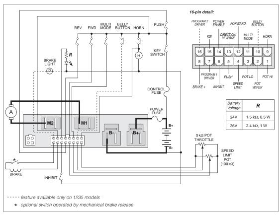
Fig. 6 Basic wiring configuration using on/off switches, Curtis PMC 1225/35 controller.
