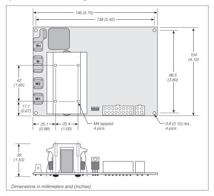
Mounting the controller via the tapped holes in the heatsink is the preferred method and requires M4 screws. If the controller is mounted via the circuit board, care should be taken to ensure that no conductive hardware overlaps the copper planes at the power connect end of the board. Additionally, at least 6 mm (1/4") clearance should be provided below the bottom of the circuit board to prevent shorts to any of the thru-hole connections.
