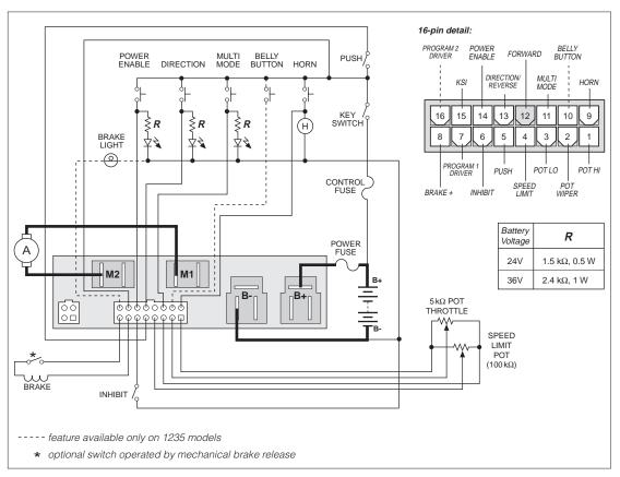
Fig. 7 Basic wiring configuration using momentary switches, Curtis PMC 1225/35 controller.
