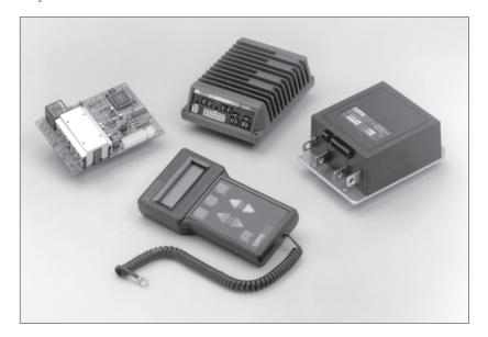
The 1223/33, 1225/35, and 1227/37 MultiMode™ controllers offer smooth, silent, cost effective control of motor speed and torque. A four quadrant, full bridge power output stage provides for solid state motor reversing and full braking power without additional relays or contactors.
