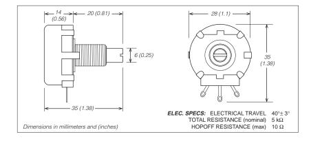
Fig. B-2 Mounting dimensions, Curtis PMC potboxes PB-5, -6, -9, and -10.
