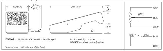
Fig. B-4 Mounting dimensions, Curtis electronic throttle (ET series).
