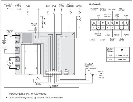
Fig. 3 Basic wiring configuration using on/off switches, Curtis PMC 1223/33 controller.
